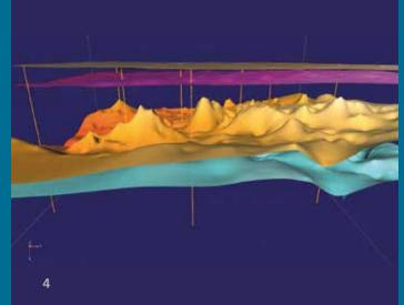
IWES' seismic and the establishment of a 3D model of the subsoil in wind park areas offer therefore a convenient flexibility in wind farm development, including rearrangements in the wind farm layout – without the need for cost-intensive geotechnical post-surveys.
