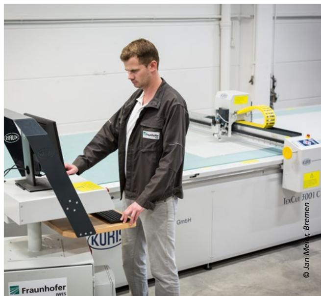
■ *A precise cutter ensures a consistent level of quality when tailoring fiber mats.*
