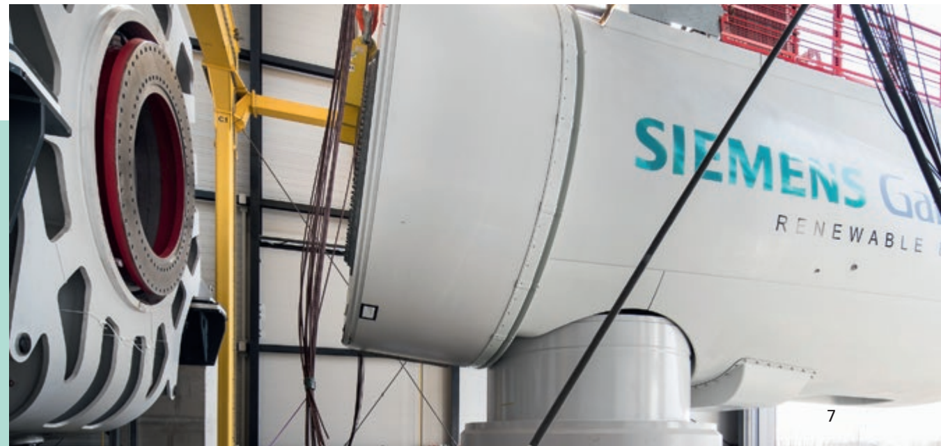
Nacelle of an 8 MW wind turbine arriving at the DyNaLab for testing
