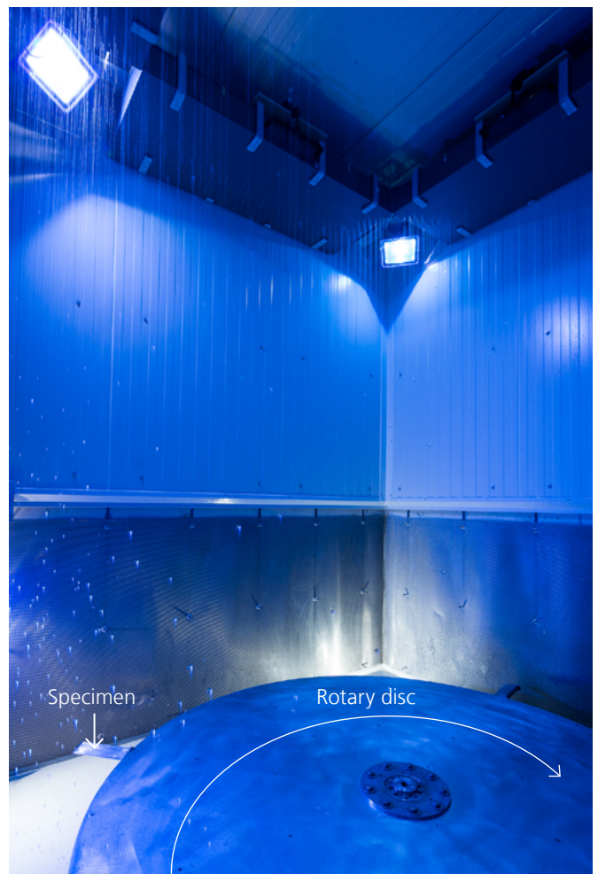
The IWES Leading Edge Lab deliver data to evaluate the resistance of rotor blade coatings to rain erosion.
