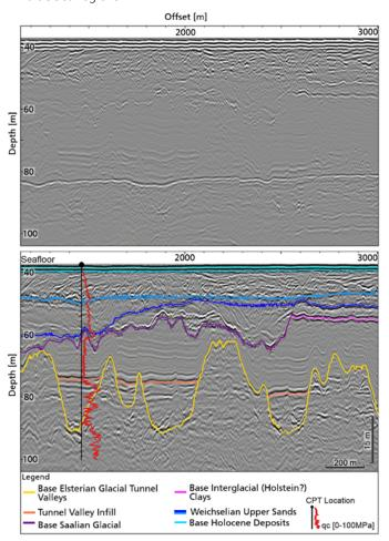
Data example from the southern North Sea showing the detailed imaging of glacial geological structures and deposits
